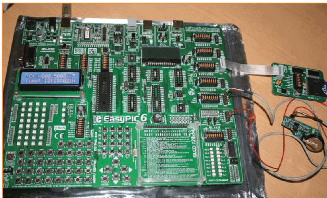
Figure 3. This how the project got developed at the author's home using a Mikroelektronika EasyPIC6 development system and some add-ons.
